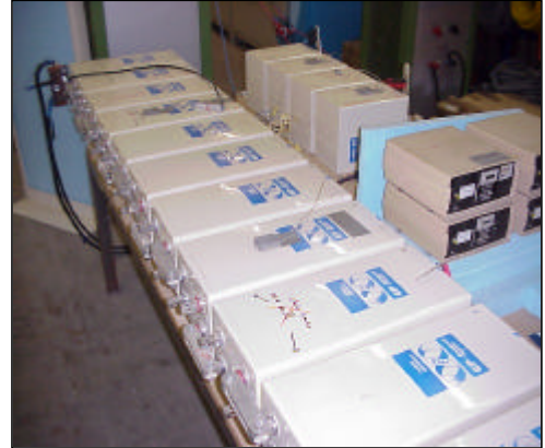
Figure 2: View of the 24V VRLA battery with one string with 12 cells 2V/550Ah (left) and one string with 4 monoblocs 6V/100Ah (background right).
